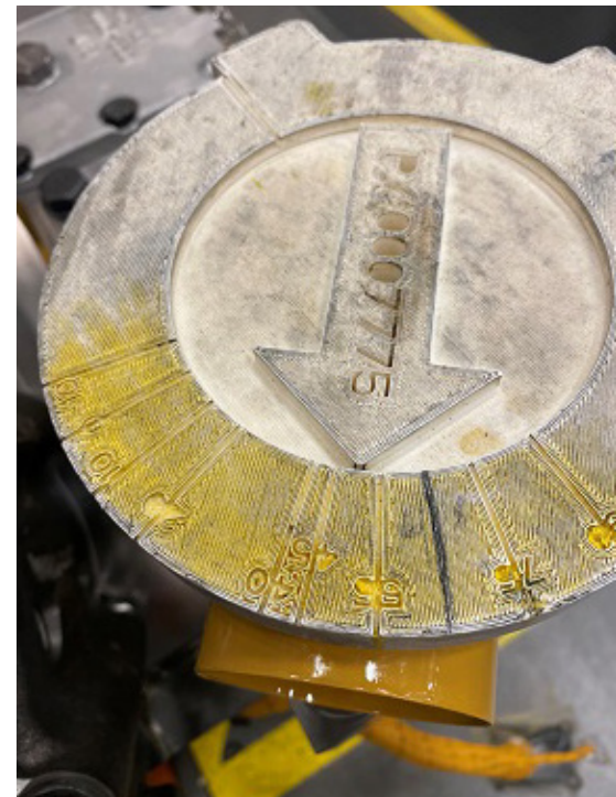
The FDM locating fixture shown on top of the breather outlet port
