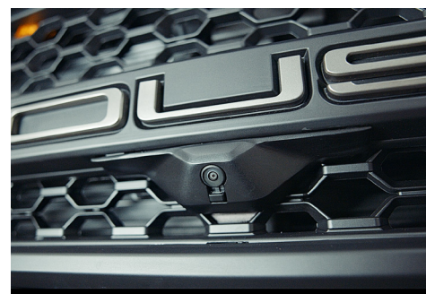
The finished camera and 3D printed bracket shown mounted to the F-150 truck grill.
