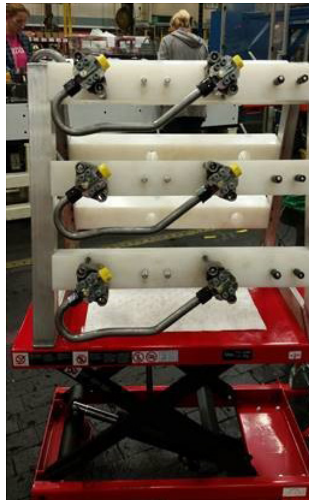
The assembly rack and one of the FDM 3D printed proof-of-concept rack components (top image).
