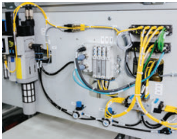
IP67-rated EtherCAT Box modules from Beckhoff are convenient for direct mounting on the USS machine. Photo credit: Beckhoff
