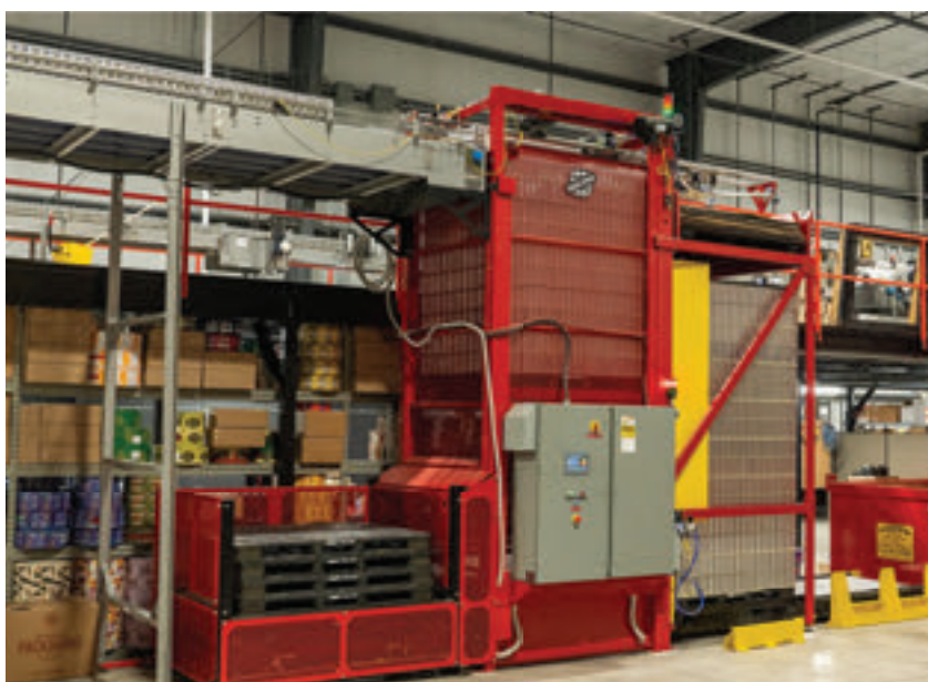
Ska Fab's Magic Bus Depalletizer is a full height automatic depalletizer for aluminum cans or metal containers on lines up to 1,000 CPM.
