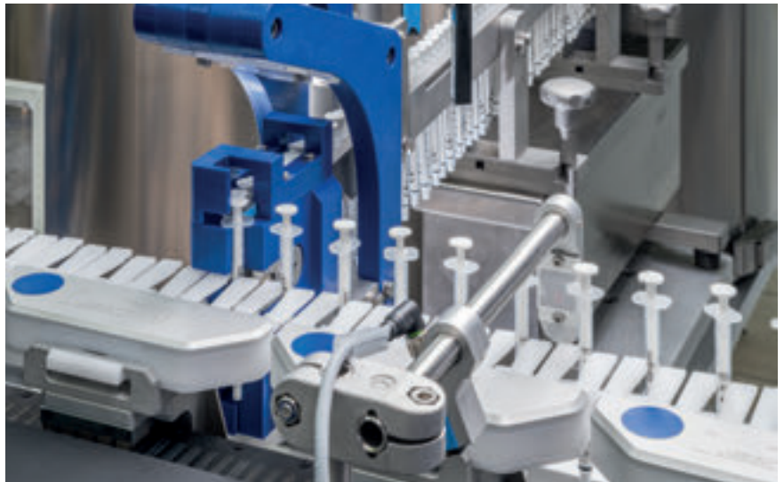
↑ Five pipettes are loaded onto one of the Beckhoff transport system's movers.
