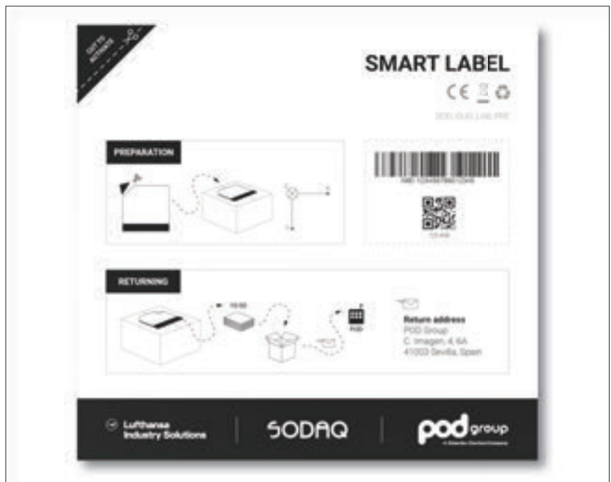
↑ The user cuts the corner of the adhesive label to activate it, places it on the box/shipment manually, and scans a barcode with a smartphone. (All images credit: POD Group)
