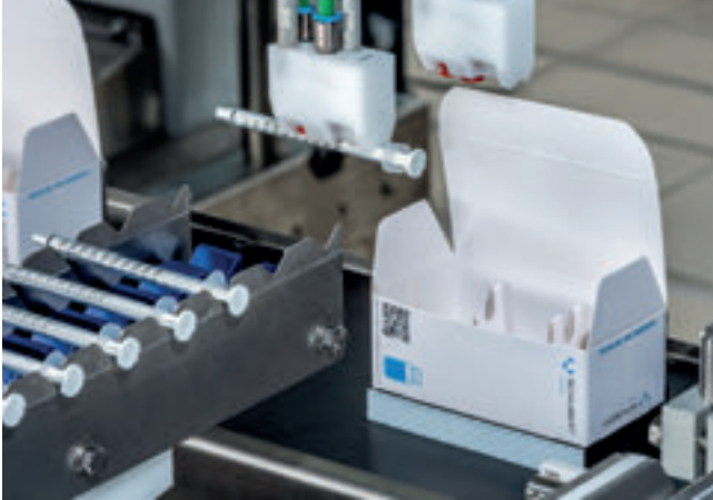
↑ Labeled vials are loaded into cartons.
