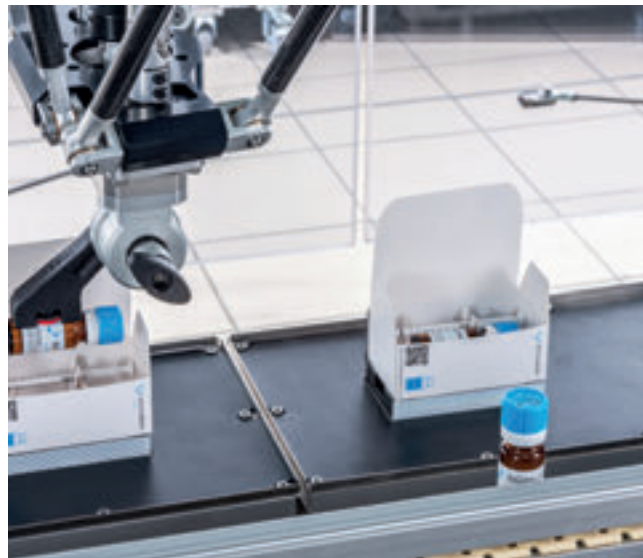
↑ A robot picks up one pipette for each carton of vials.
