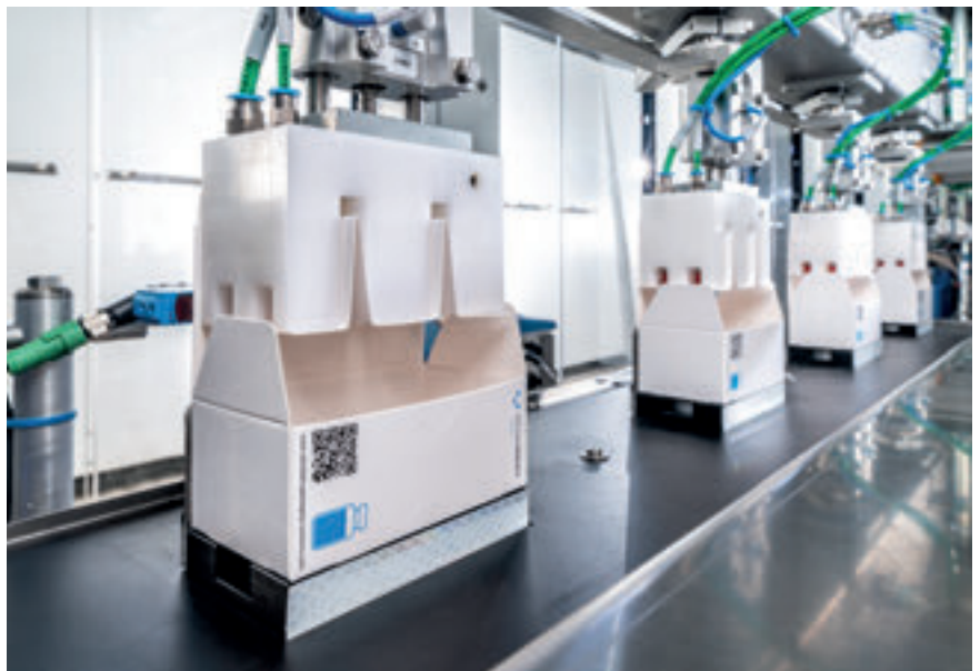
↑ Schubert developed a format-part-independent forming process for the partitions.
