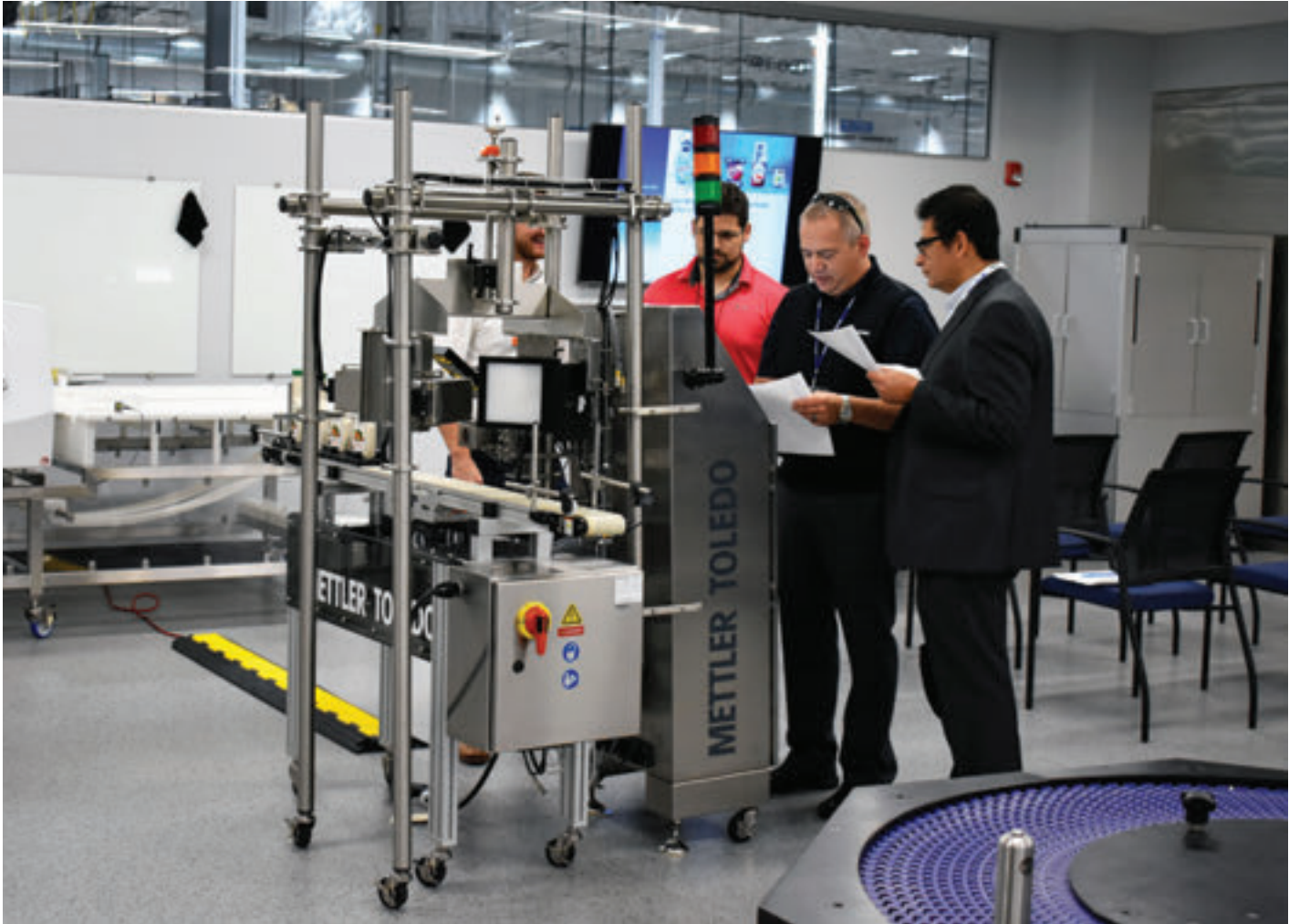
The V31 vision machine in the onsite Applications Center. Here, customers can send in test products to receive a test report of the system's performance and capability prior to purchase.
