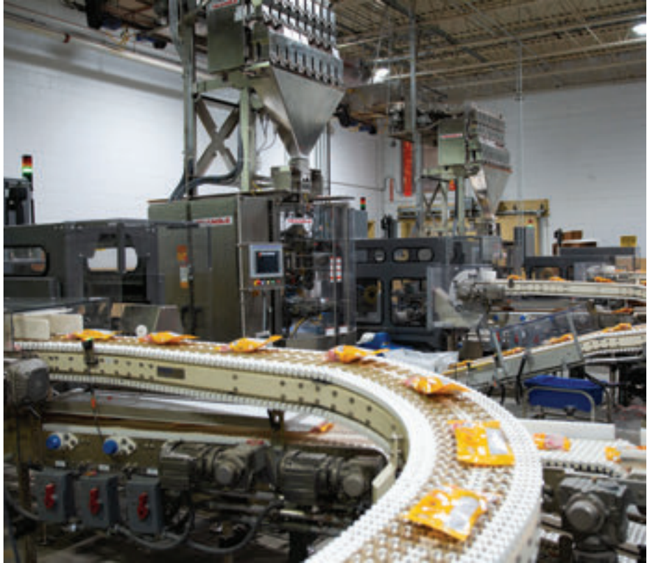
The Triangle inline combination weighers weigh the twist Caramel Creams and then they are bagged. Filled bags are moved via conveyors to Fallas Automation case packers.
