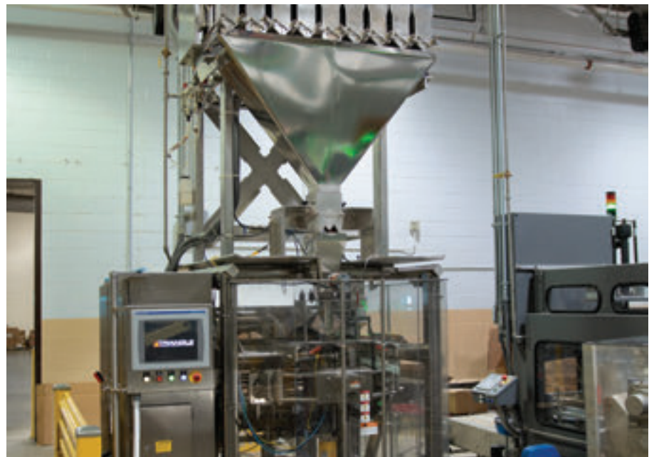
In 2021, Goetze's Candy replaced a bagging machine it had since the early 1960s with this Triangle vertical form fill seal (VFFS) bagger.
