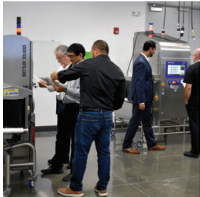
The X33 (left) and X36 (right) X-ray Inspection Systems in one of five factory acceptance test rooms at the Lutz facility. Customers are able to witness and perform tests of their machines prior to shipment.
