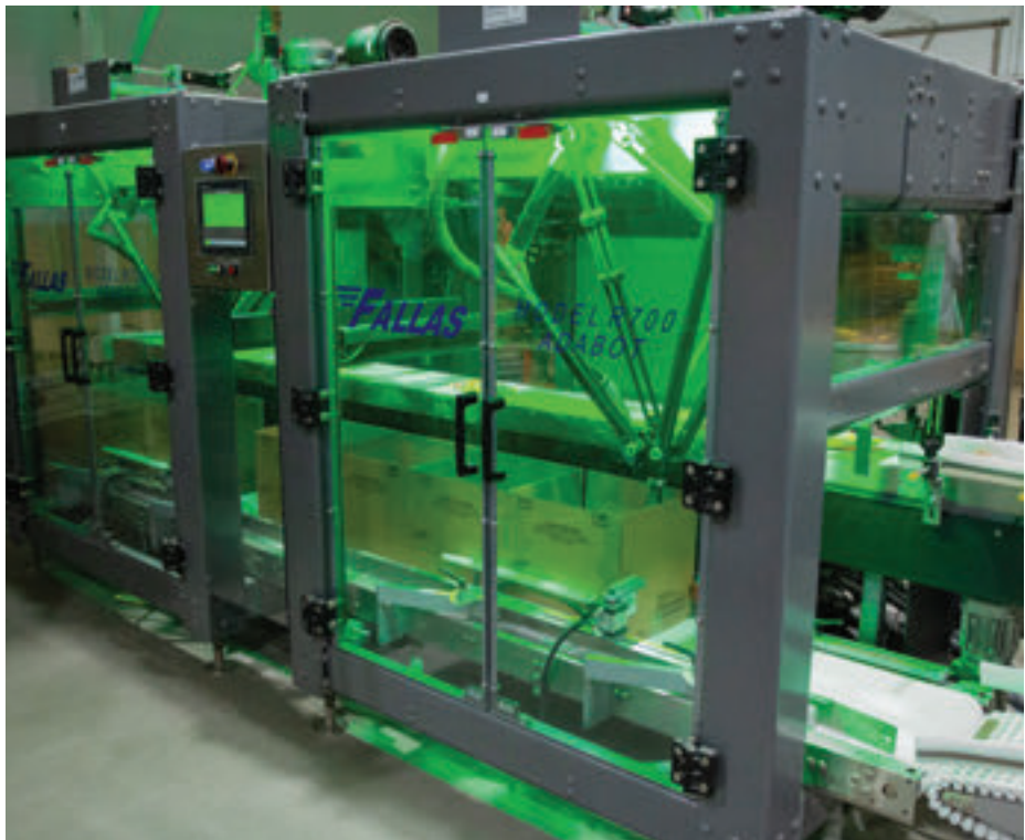
After product goes through the Fallas Automation case packer, it is transported to robotic palletizers.
