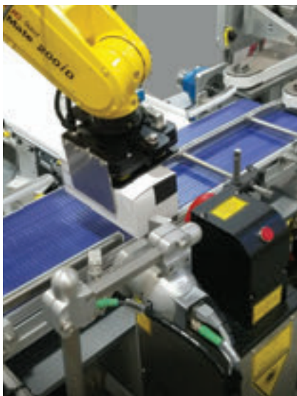
↑ Videojet and ESS worked together to ensure the carton arrived at the coder in the right orientation. (Image credit: ESS Technologies, Inc.)
