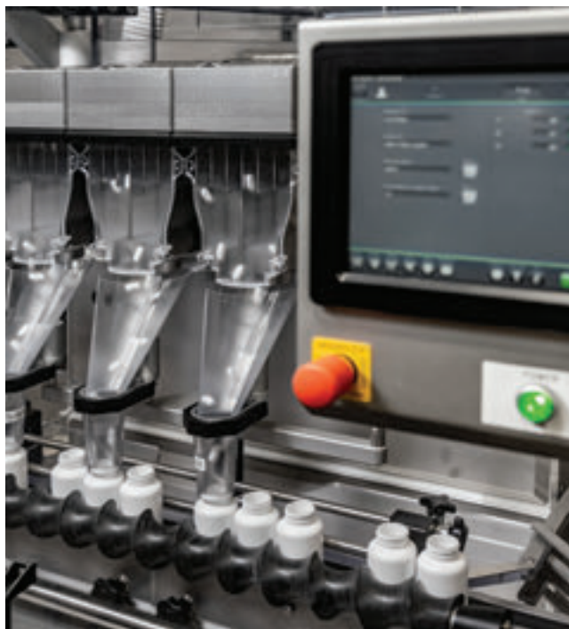
↑ The Cremer 622 tablet counter is currently equipped with three fill heads.
