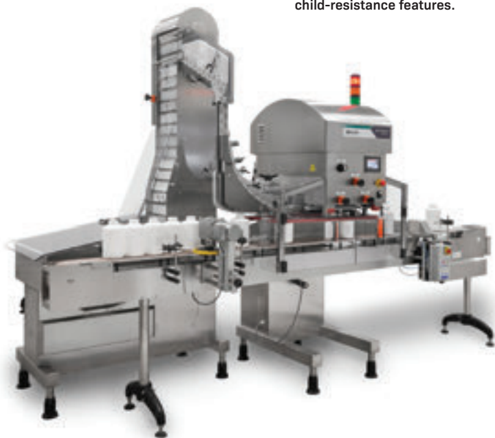
↑ The Cremer 622 tablet counter is currently equipped with three fill heads.
