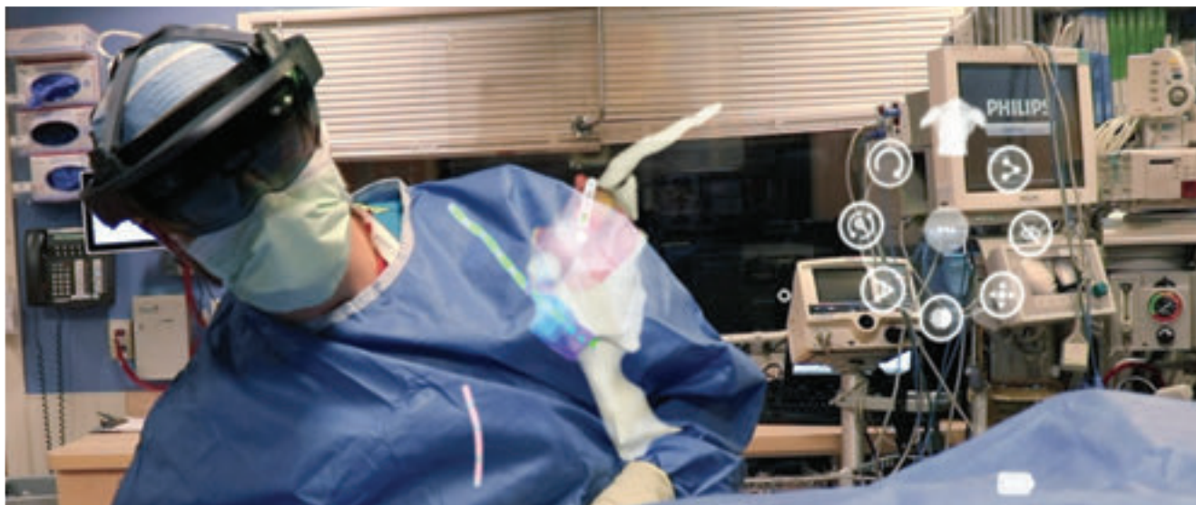
The SentiAR Wearable Command Center is an interprocedural augmented reality (AR) system—with the user interface built off the Microsoft HoloLens—that enables the electrophysiologist to model the heart. (Credit: HS Design, Inc.)
