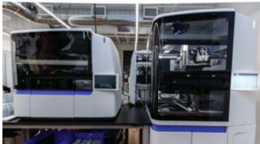
↑ Selux Diagnostics, Inc. pivoted from a tabletop version (left) to a floor-standing, two-floor system (right) based on user feedback. (Credit: Selux/HS Design, Inc.)
