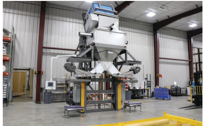
↑ The integrated process MTS came up with includes a crusher, a scale system, and customized feeder and controls required to report diagnostics to the vaccine manufacturer operating the system.
