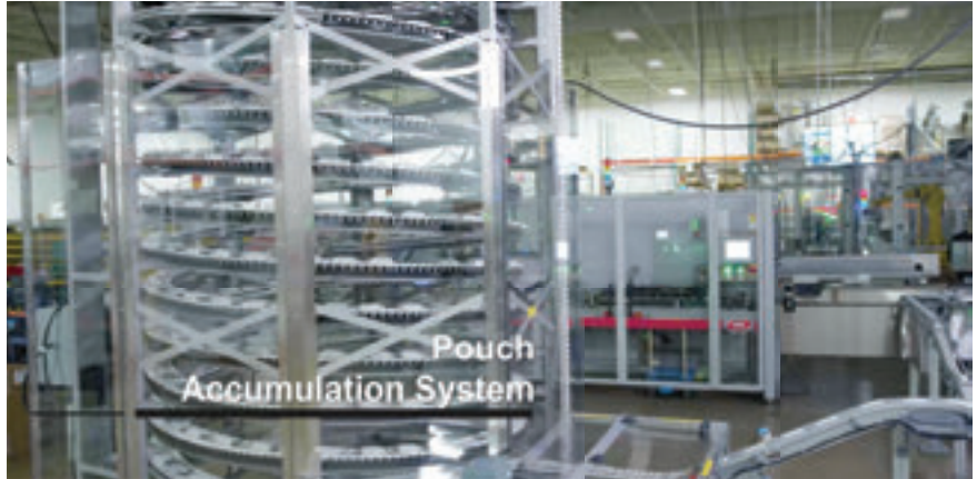
↑ The Ambaflex Pouch Accumulation Module provides a buffer of material to absorb the imbalance in product flow.
