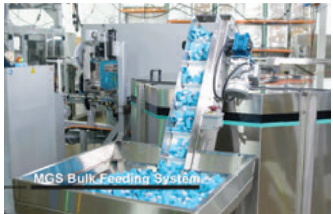
↑ Prior to the MGS assembly module, bulk actuators are dumped into a hopper; a centrifugal bowl is utilized to singulate and orient them.
