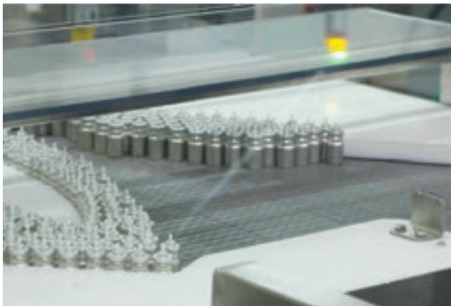
↑ Depalletized canisters are oriented for automated processing.
