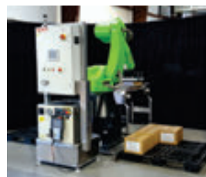
Mini Cell-E with Collaborative Robot
