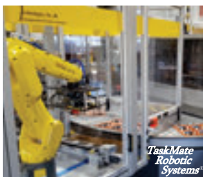
Loading a Blister Packaging Machine
