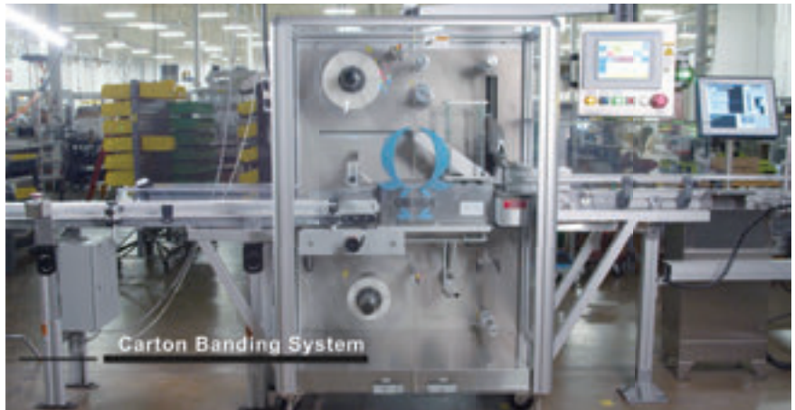
↑ The Omega Stretch Banding Module combines serialized cartons into one stretch wrapped bundle.
