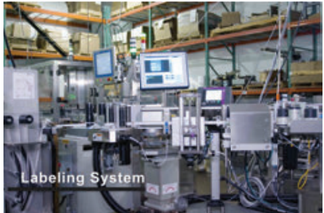
↑ The Canister Labeling Module from Accraply applies labels with product information onto each canister.
