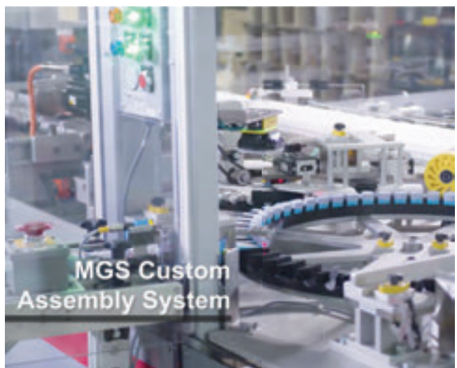
↑ Linear servos insert the canisters into the actuators when the components are properly aligned in the starwheels.
