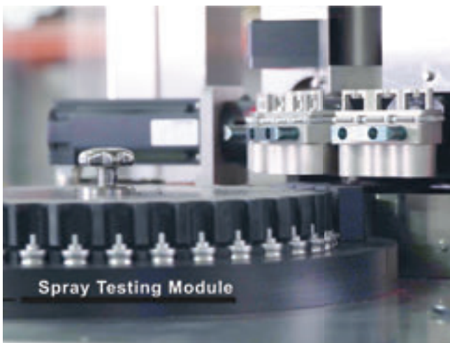
↑ The Brooks Machine & Design Spray Testing Module primes and tests each individual canister for proper discharge.
