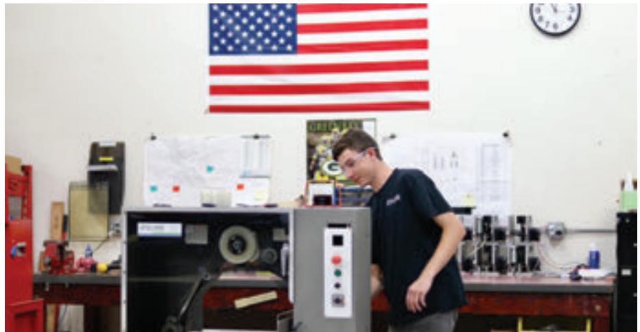
Felins also manufactures the Flex-Strap machine, a stretch film banding system that bundles a wide range of products, especially products in the manufacturing and wood industries.
