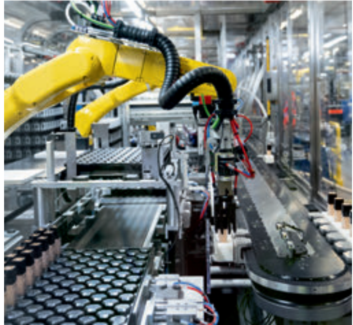
EtherCAT provides the optimal fieldbus for synchronizing robotics with mechatronics, like the XTS, which can replace robotic functions in some instances. Photos courtesy of: Beckhoff Automation
