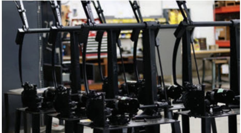
Machine frames for the Felins Pak-Tyer, a semi-automatic tying machine, await assembly.
