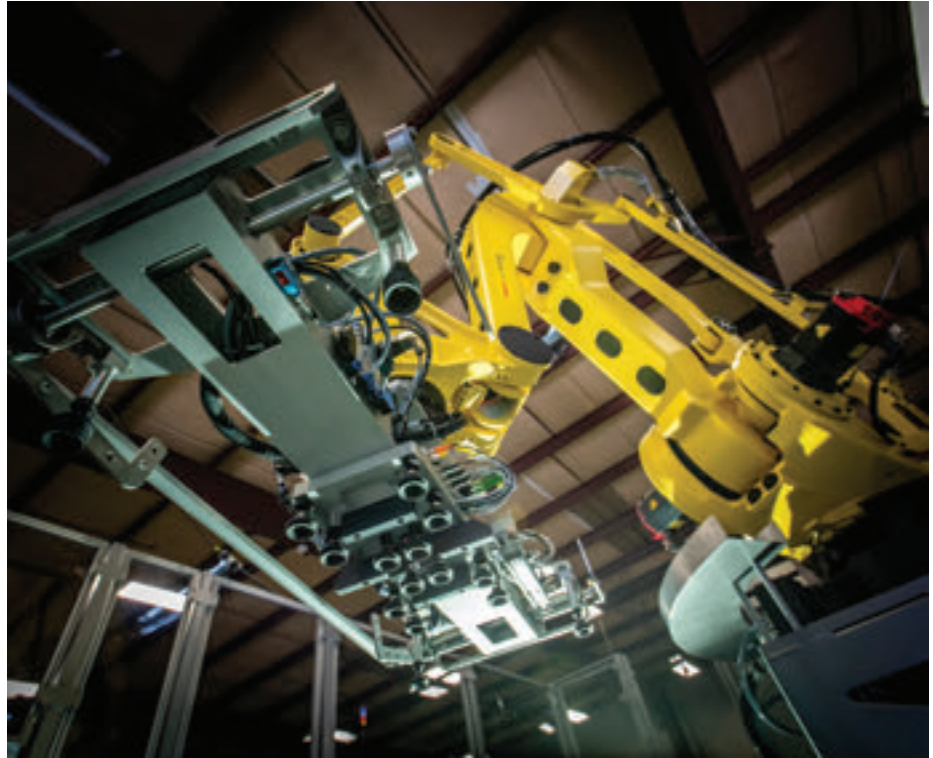
Serpa’s pharmaceutical robotic palletizer with custom end of arm tooling.
