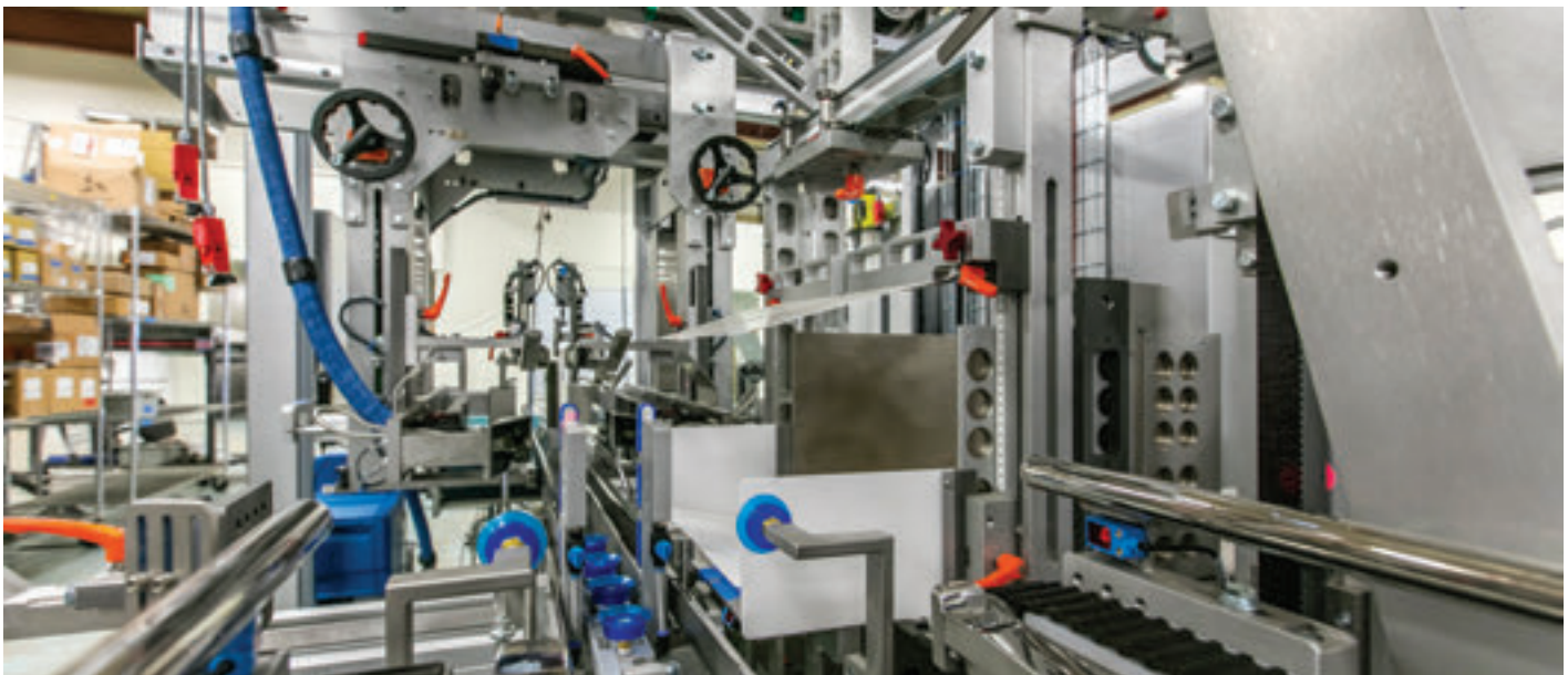
The inside of a Serpa case packer being assembled on the OEM's floor.
