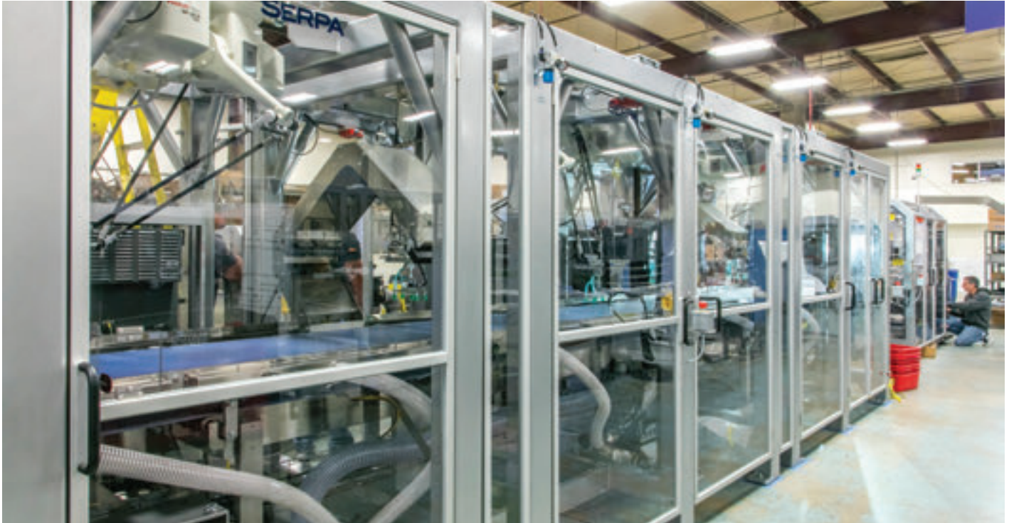
This is Serpa's P150 intermittent cartoner which features a balcony design that provides maximum access to all of the drive components from one side of the machine.
