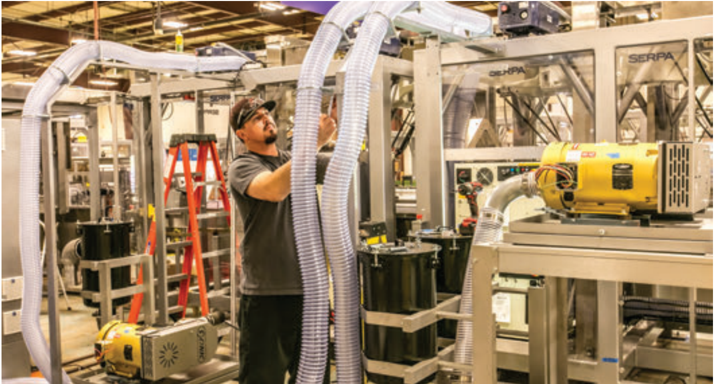
Scott Pitchford, a mechanical assembly technician, works on the vacuum collator system for a cartoner.
