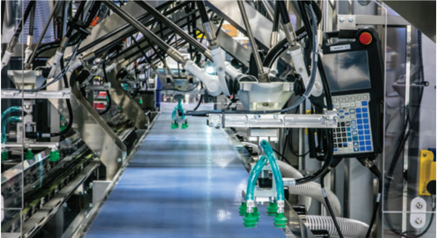
Spider robots sit atop a conveyor on one of Serpa's intermittent cartoners.
