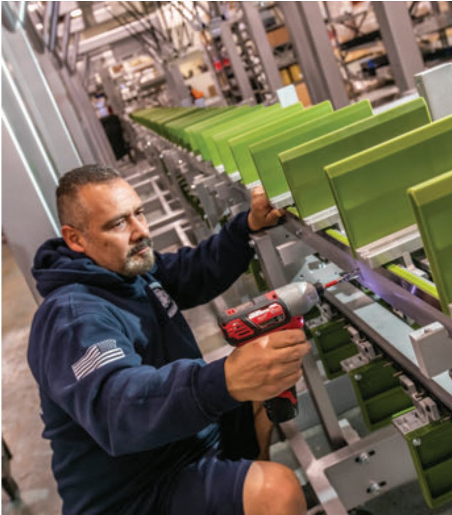
Aurelio Lara, a mechanical assembly tech, works on the product bucket conveyor for a cartoner.
