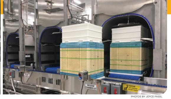
After crumbling 40-lb blocks, a larger capacity line forms and produces a homogenous 640-lb block using seven state-of-the-art vacuum chambers manufactured by Loos Machine & Automation.
