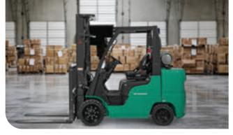
injection system, the engine enables high levels of torque and horsepower, while maintaining compliance with all CARB and EPA emissions regulations. The forklifts are available with a 7,000- to 8,000-Ib capacity.
