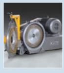
accelerates bulk material entering the central inlet of the opposing stationary disc. As material travels from the center to the periphery of the discs at high speed, it passes through a path of five intermeshing rows of rotating and stationary pins, with the desired tight particle size distribution obtained by controlling the rotor speed.
