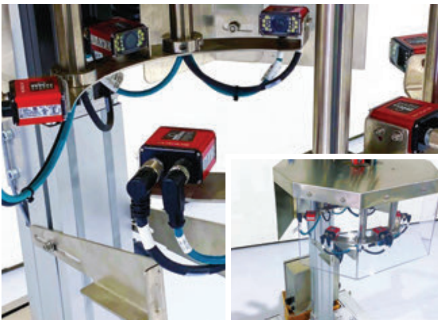
↑ The compact machine adds no more than 34 in. to the length of a packaging line. It reliably inspects all angles of the bottle or label at speeds up to 100 bottles/min.
