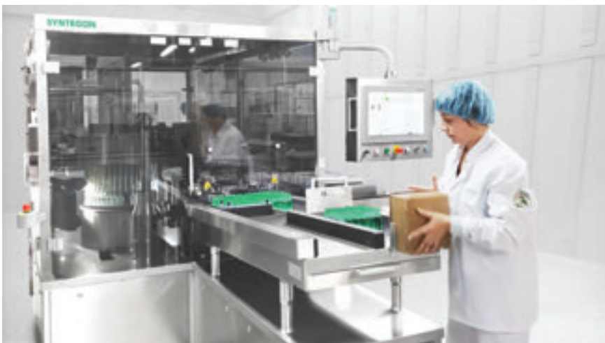
↑ The system allows for contactless handling of glass containers without mechanical stress.
