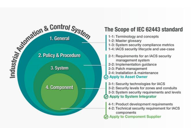
**The IEC 62443 guidelines define four security threat levels.** The security standard level 2 is the baseline requirement of the automation industry. It relates to cyber threats posed by hacking, which is the most common attack experienced by system integrators who secure industrial networks. Level 1 is to protect against accidental unauthenticated access and Levels 3 and 4 are against intentional access by hackers who utilize specific skills and tools.
