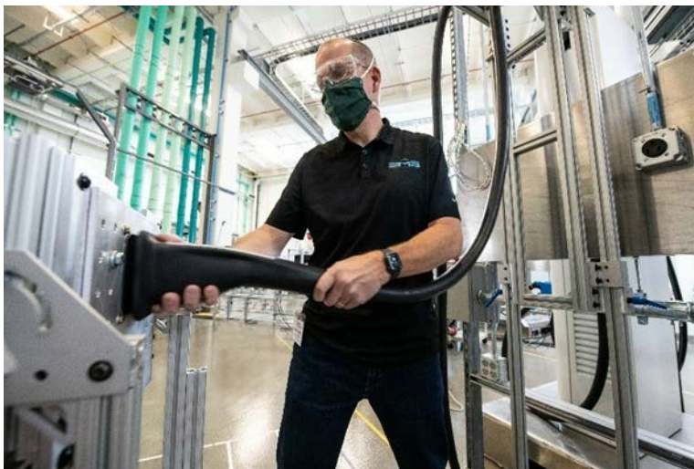
Figure 1 Ergonomic and Fit Tests of Megawatt Charging System Connectors
