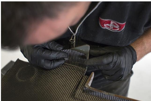
In addition to the need for expensive up-front tooling in the form of molds used to shape parts, the process - as the name suggests - is done almost entirely by hand, with technicians manually cutting material to size and pressing it into molds.
