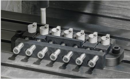
Designed to hold lock barrels in place during a secondary reaming, this part must be very stiff to tolerate the forces and vibration of the reaming tool. The rapid turnaround of Fiber™ means this part can be produced overnight, while the toughness of composites result in a part with material properties similar to aluminum.
