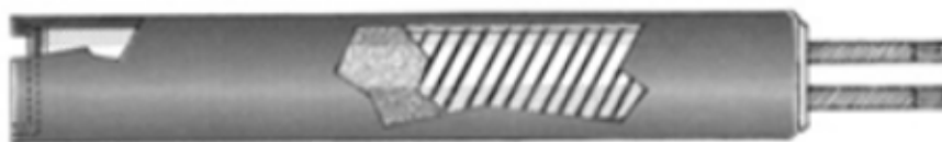
Figure 2: Swaged cartridge heater. Source: Backer Hotwatt
