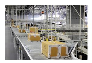
shuttle system to a goods-to-person workstation, then handled once to fill store replenishment and direct-to-consumer orders. This system combines retail and customer orders at each workstation, enabling one person to process items eight times faster than they would at a typical distribution center.
