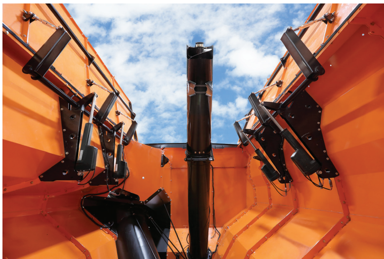
Smart electromechanical linear actuators, such as the four Thomson Electrak ® HD units shown here, help engineers design machines with components that communicate with each other and operate without the need for manual interaction.
