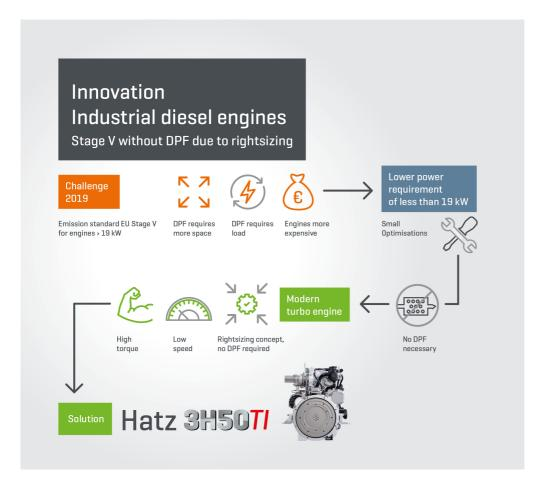
For the use of somewhat smaller engines of less than 19 kilowatts, only minor adaptations are required in the specifications of the machines.
