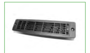
Vector nozzle for ideal windshield defrosting
