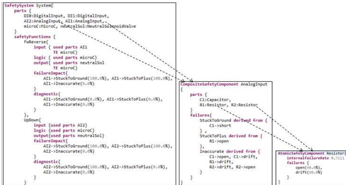
Figure 3: componentized failure specification using a textual DSL
