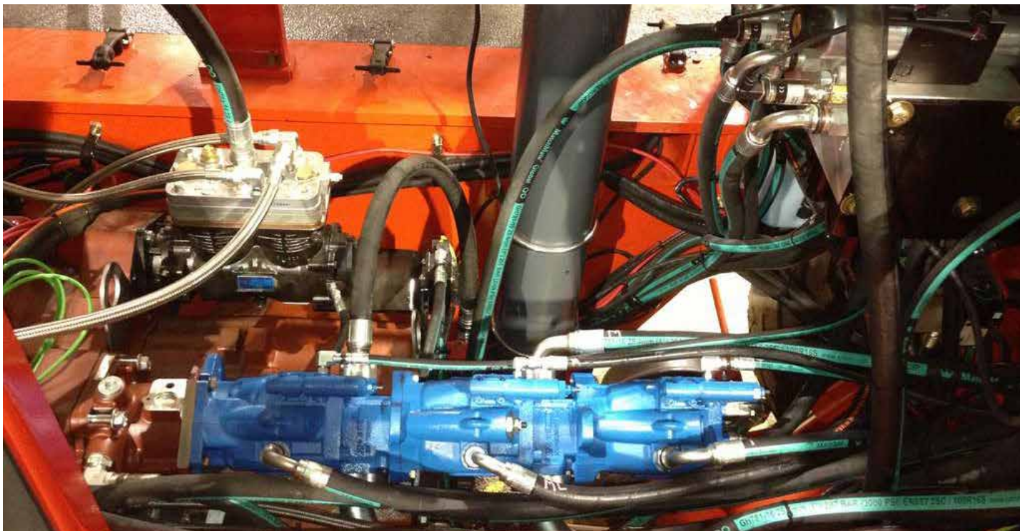
Eaton's 420 series pumps fit within the system's space constraints and provided more power and increased efficiency in the triple pump configuration.
