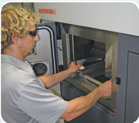
Directed's Erling LaSalle prepares an additive metal manufacturing machine for its next build cycle.
