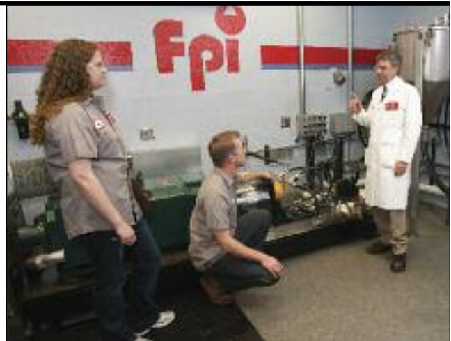
200 HP dynamometer with electrical regeneration capabilities used for testing energy efficient fluids.
