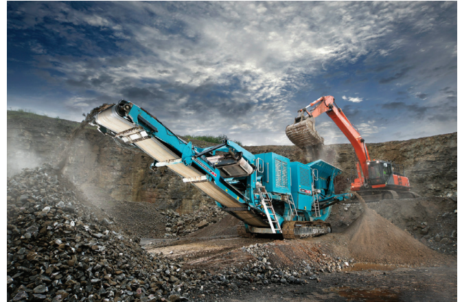
Terex stone crusher powered by Scania 9-litre industrial engine Great Britain Photo: Bryan Winstanley 2011
