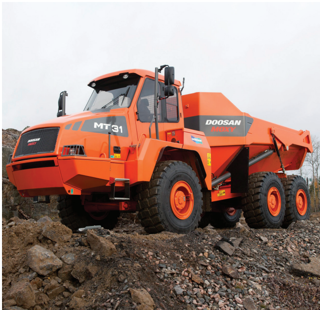
Articulated Dump Truck (ADT) from Doosan Moxey, powered by Scania 9-litre industrial engine. Stage IIIB/Tier 4i compliant.
