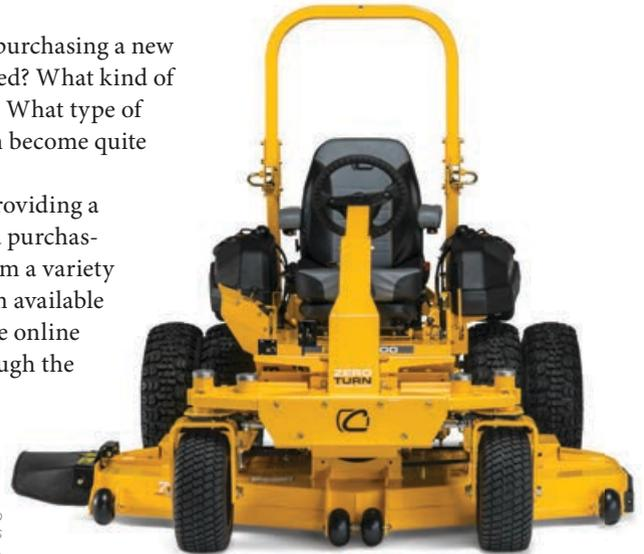
*The Cub Cadet PRO Z 972 SD zero-turn allows you to comfortably mow a straight line, execute zero-degree turns and operate on a hillside with up to a 25-degree slope.*
