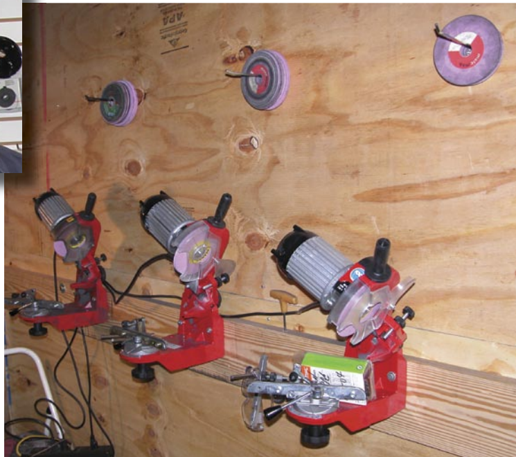
A chain grinding station is designed to reduce technician downtime (grinding chain) by 25%.
