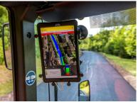
operators, project supervisor and site managers can monitor and track all compaction values in real time.
