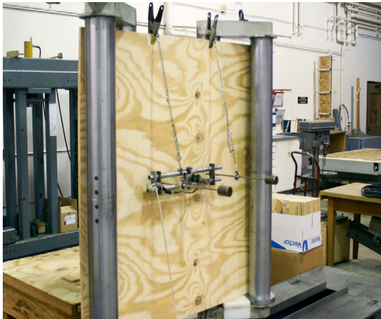
Plywood panel flexure testing at APA's Tacoma research laboratory.
