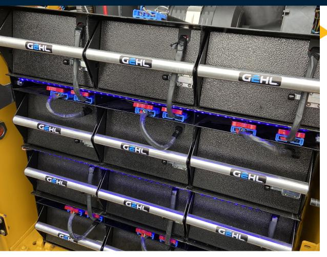
GEHL'S CONCEPT 165E ELECTRIC COMPACT SKID LOADER, FEATURED AT CONEXPO-CON/AGG 2020, INCORPORATES 12 REMOVABLE BATTERY PACKS, WEIGHING 48 LBS. EACH, WHICH CAN BE EASILY REMOVED, REPLACED AND RECHARGED AS NEEDED.
