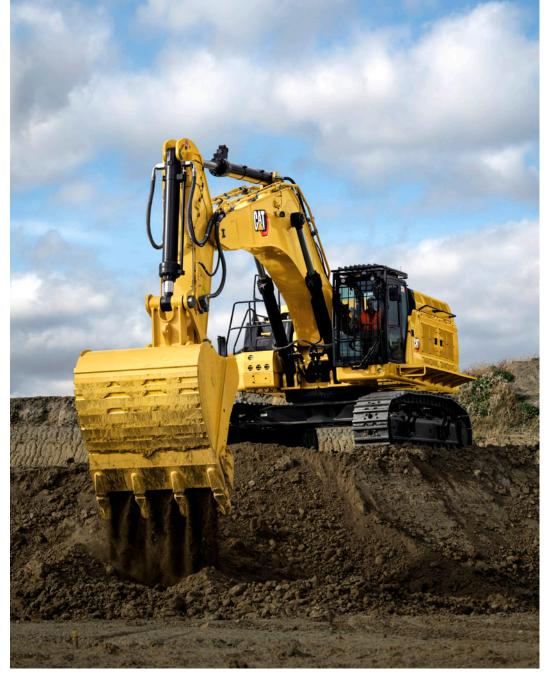
cylinders. To expand productivity, a dedicated swing pump aids multifunction capability and provides 10% more swing torque. Cat Payload, upgradeable Cat Grade with 2D, Lift Assist, 2D E-Fence, Auto Hammer Stop and Cat Product Link are standard.
