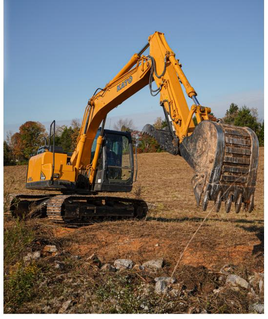
by a 105-hp Isuzu Tier 4 Final diesel engine and have a 73-gal. fuel tank. They include a quick-response fourpump hydraulic system with dual auxiliary hydraulics. The ROPS/TOPS/FOPS pressurized cabin has centralized switches, a 7-in. LCD color touchscreen monitor with standard side and rear camera feature and retractable windshield. Large covers and a large-capacity tool box enable ease of service.
