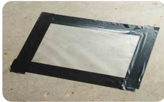
The first step in the Rubber Mat Test is to tape and seal a rubber mat or polyethylene sheet to the concrete surface for 16 hours or more.
