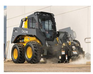
models is the Anti-Stall feature that monitors the engine load to quickly prevent the engine from stalling. This allows the operator to use the maximum horsepower efficiently when pushing large amounts of material.
