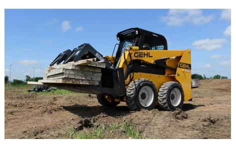
Gehl's hydraulic systems boost productivity by using some of the top technology combined with innovation. Hydraulic component efficiencies have improved through the years, allowing the machines to do more with small engines without sacrificing power. They consume less fuel and operate quieter than machines of the past. For maximum power, the range goes up to what is reported to be the largest skid steer in the market, the V420, which offers 120 hp and a rated operating capacity of 4,200 lbs.
