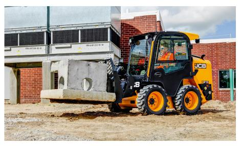
Engine advancements in skid-steer models have resulted in engines that produce enhanced torque and horsepower while using less fuel, making them more efficient than previous models. In addition, electrohydraulic controls have improved machine efficiency, allowing the main control valve to be powered by electric signals instead of servo hydraulics.
