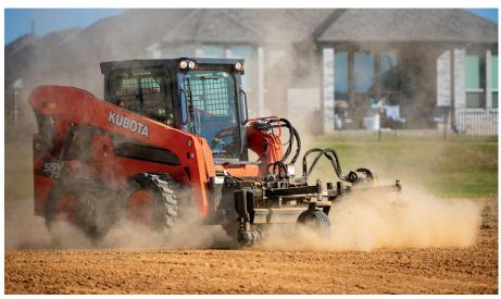
The SSV Series is powered by a Kubota Tier 4-certified, four-cylinder diesel engine and features standard two-speed travel and optional high-flow hydraulics. Borrowed from the company's compact track loaders, the proven loader arm design with vertical geometry can push and dig as well as a radial machine. It is reinforced in all the right areas, including critical connections to the coupler and rear crossbar.
