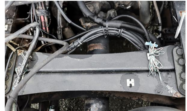
Body Builder Hydraulic and Electrical Routing
