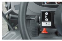
If the forward/reverse lever is not in neutral (N), the engine cannot start.
