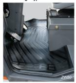
The walkthrough type cab allows for easy access from either side. The flat floor enables easy cleaning.
