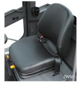
The short-stroke suspension seat is provided as standard equipment to absorb shocks and vibration during operation, reducing operator's fatigue in long hours of operation.
