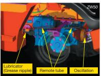
Remote easy access lubrication and engine oil drain.
