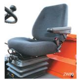
A long-stroke suspension seat, which absorbs shocks and vibration well, is standard.
