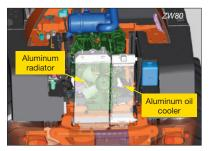
The aluminum radiator and oil cooler are located side by side for easy cleaning.
