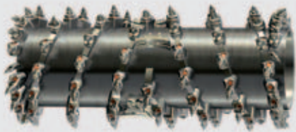
ECO cutter Milling width: 7 ft 3 in (2,200 mm) Milling depth: 0-14 in (0-350 mm) Tool spacing: 1 in (25 mm)
