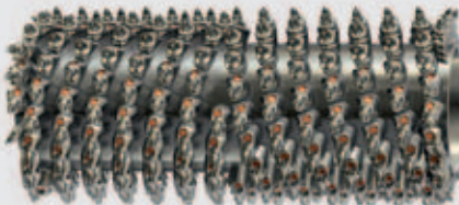
Fine milling drum Milling width: 7 ft 3 in (2,200 mm) Milling depth: 0-4 in (0-100 mm) Tool spacing: \frac{5}{16} in (8 mm)
