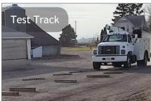
Sometimes it's more about "where" you need to work that "what work you need to do." An important test for our new TMAX Aluminum mechanic body was our test track. We loaded shelving and side pack compartments to the max, had our technician run through a test track full of 4x4 and 6x6 timbers to simulate the tough environment our equipment often encounters.
