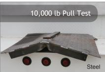
The exclusive extruded aluminum top on the Stellar® TMAX™ Aluminum mechanic body was designed, tested, and proven to meet or exceed the strength of our steel compartment tops. Plus, we pull tested a single mounting bolt in our mounting rail hardware to 5000 lbs. before it failed, which means 20,000 lbs. for a common four bolt mounting pattern. Proven to succeed.
