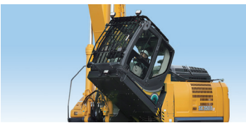
Tilting cab This picture is from different model Tilting cab is standard.
