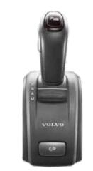
When steep-grade startability and low-speed maneuverability are critical, the I-Shift with Crawler Gears is the answer for maximum GCW loads. The crawler option adds either one or two gears to I-Shift, a low gear and ultra-low gear, for low-speed control.
