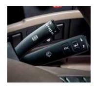
The intelligent Volvo Engine Brake (VEB) is an enhanced engine braking system that gives drivers precise control over engine braking, and saves the truck's brakes for when they're needed most. The result is phenomenal retarding horsepower at low rpm, where the engine spends most of its time and where braking is needed most. An impressive 600 hp of retarding is available at 2200 rpm with the D16.
