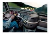
I-See. Combine I-Shift with an intelligent cruise control and you get I-See. It's a unique system that learns the topography of the road. Later on, it automatically uses its knowledge to save fuel when the intelligent cruise control is engaged.
