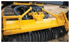
SELF-POSITIONING DEFLECTOR. The patentpending self-positioning thrown object deflector helps direct thrown material at a consistent discharge angle, regardless of head position.
