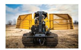
**SERVICEABILITY.** A center-mounted cooling package is easy to access, and two large hinged doors swing open to expose the engine compartment for maintenance without additional tools.
