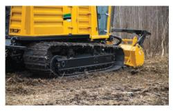
TRACK OPTIONS. With the option of either steel or low ground pressure (LGP) tracks, operators can choose which style fits their jobsite needs. With the weight of the mulcher head calculated in, the total machine weight is centered on the tracks resulting in even weight distribution and lower ground pressure.
