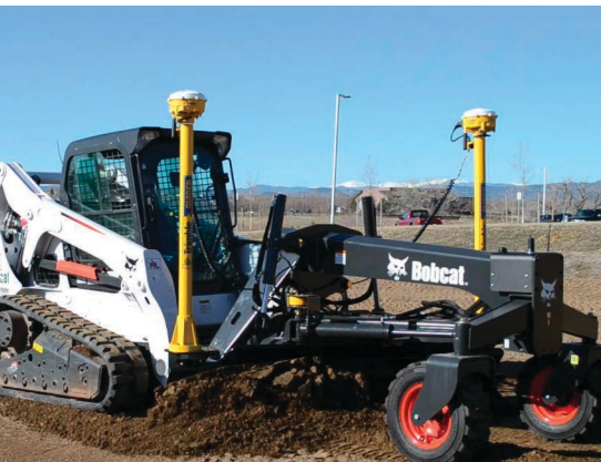
Bobcat with HD Grader Attachment and Trimble GCS900 Grade Control System with Dual GNSS
