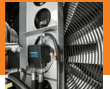
■ A reversing fan back-blows cooler cores to reduce debris buildup and increase uptime.
