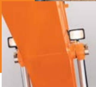
Cab-mounted lights, two boom-mounted lights and a rearview camera provide excellent job site visibility, regardless of when or where you work.
