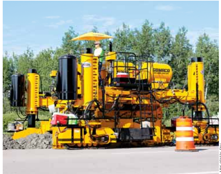
The Smart Pivots and Smart Track Rotation now let the G+ system automatically control the direction and speed of track travel through a radius.
