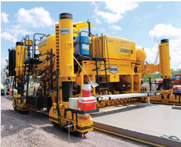
The GP3 offers a 42 inch (1067 mm) hydraulic leg height adjustment along with a manual leg adjustment of 36 inches (914 mm).
