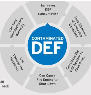
**DEF CONTAMINANTS | Copper, Zinc, Chromium, Nickel, Iron, Aluminum, Phosphorous, Magnesium, Calcium, Sodium, Potassium.**
