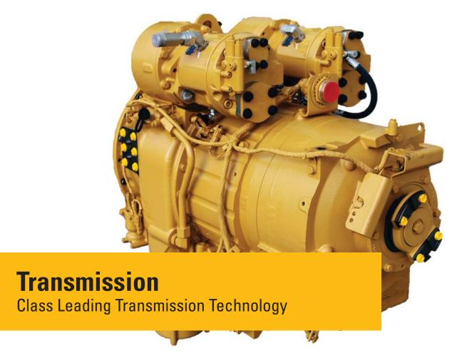
The Cat TH31 six-speed forward, single speed reverse transmission features Advanced Productivity Electronic Control Strategy (APECS) and Electronic Clutch Pressure Control (ECPC) which deliver smooth gear changes with improved acceleration and higher productivity.
