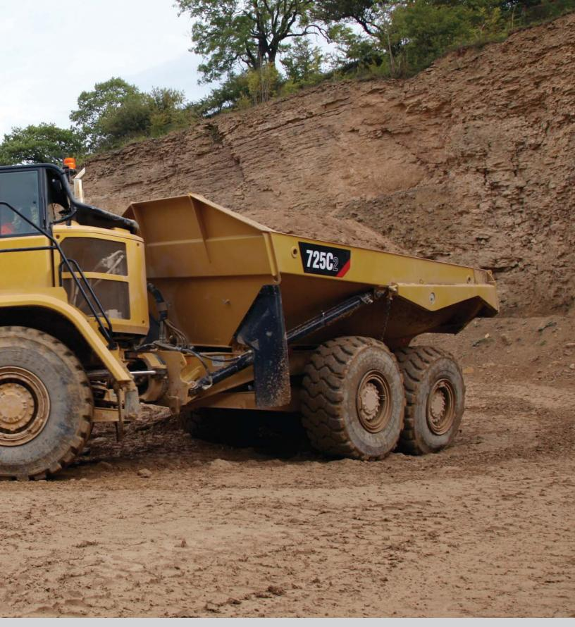
The Cat 725C2, with a 15  $\rm m^3$  (19.6  $\rm yd^3$ ) 24 tonnes (26.5 tons) capacity, offers proven reliability, durability, high productivity, superior operator comfort and lower operating costs.
