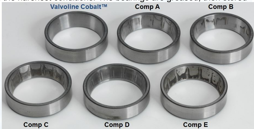
Figure 7: Bearings from 100% Synthetic Sea Water Corrosion Testing
