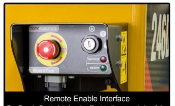
The Remote Enable Interface is affixed to the rear exterior of the machine. It contains the key switch used to enter/exit remote control and pairing modes. It also contains the Service and Ready LED indicators and an Emergency Stop Button.
