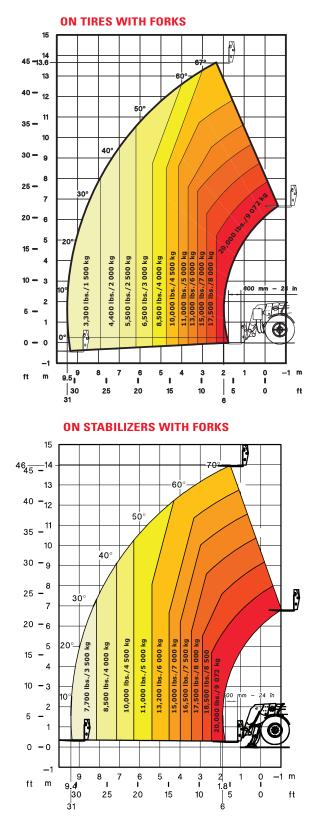
MHT 1490 load charts based on 24  $^{\prime\prime}$  (600 mm) load center per ANSI/ITSDF B56.6
