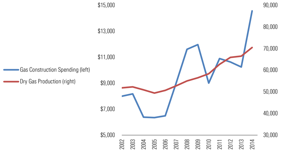
Exhibit 20. Construction Spending on Gas Infrastructure Steadily Grew to Support Rising Production Gas construction spending in millions of current dollars and dry gas production in MMcf per day
