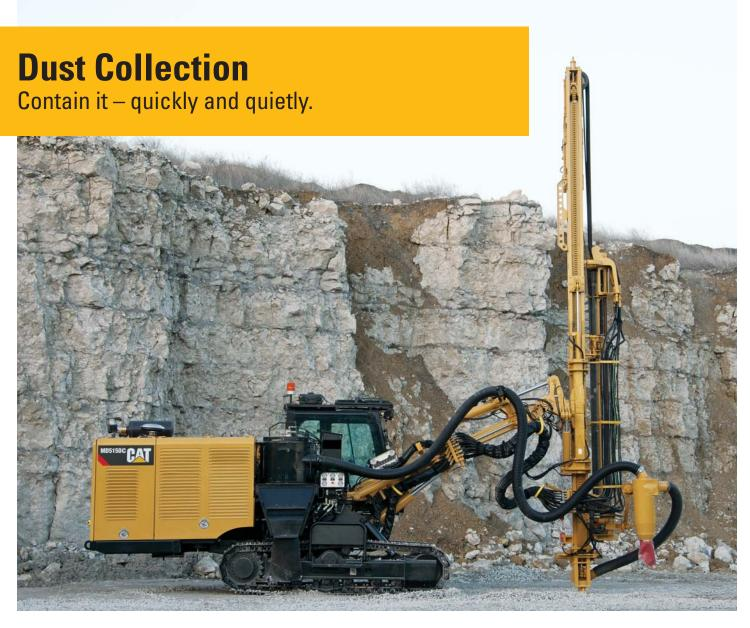
Powered to clean holes from 101.6 mm (4.0 in), the MD5150C dry dust collection system is efficient, quiet and it consumes less power than traditional dust collectors. The heavy-duty system effectively manages rock fragments and dust yet is also easy to clean and service.
